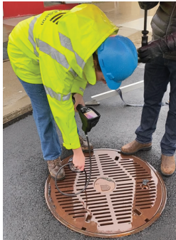
Figure 8.1 Inserting the probe into the test area.
